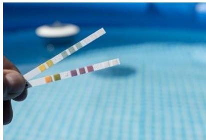
*Pool test strips are a handy tool for monitoring pool chlorine levels and pH*
